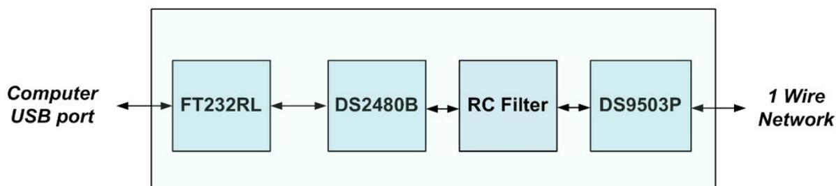
**Figure 3.** Block diagram when RC filter is on
