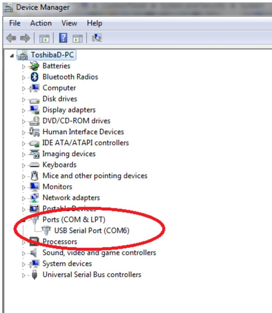
If it is necessary the com port number may be changed to lower (for example COM2, COM3, COM4) because some software applications do not work with higher com port numbers.
