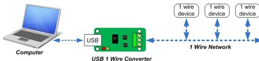
**Figure 1.** Connecting One Wire network to computer USB port
