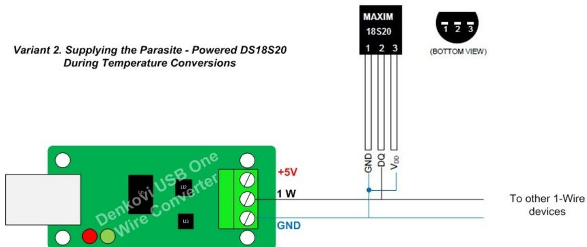
2. Connect the converter to the computer USB port. Once the device is recognized, its drivers must be installed. If this is not done automatically the drivers must be downloaded manually. Its chip set is FT232RL based, so the drivers must be downloaded from here: <http://www.ftdichip.com/Drivers/VCP.htm> and after that installed. For installation guides - <http://www.ftdichip.com/Support/Documents/InstallGuides.htm>
